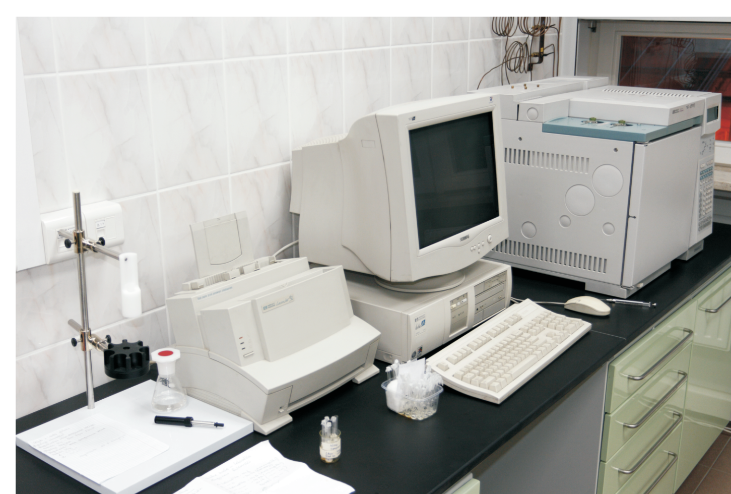
Photo 3. Hewlett-Packard 6890 GC with FID detector
