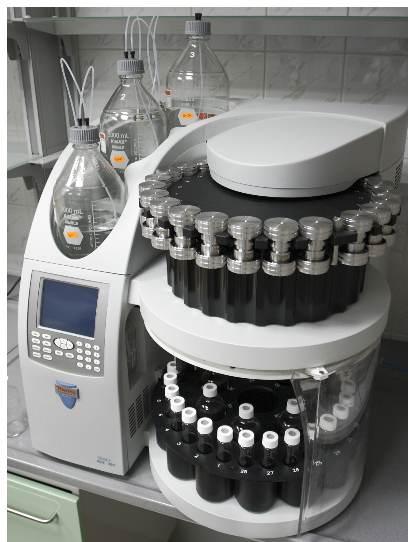
Picture 1. Accelerated Solvent Extractor – ASE™ 350 (Thermo Scientific™).
