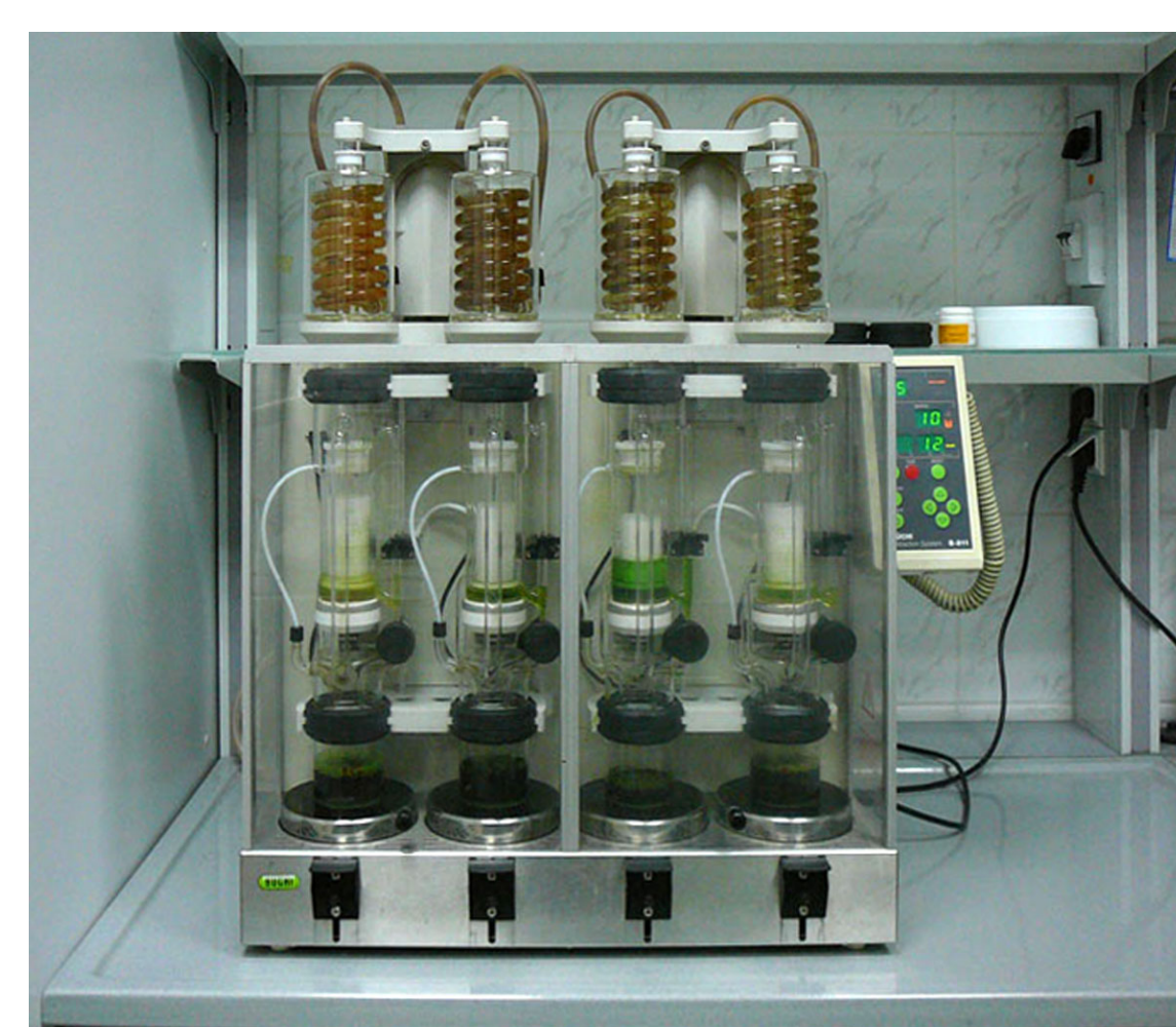
Photo 4. Extraction in B-811 Extraction System (Büchi apparatus)
